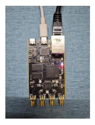
Wait for about half a minute to complete the startup process. As shown above, the normal phenomenon is that the white and red LEDs are always on, the blue LED flashes, and the Ethernet port light flashes. If the phenomenon is abnormal, please check if the previous steps were correct. The most common problems are as follows:
